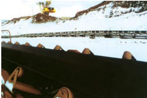
This belt can be supplied in cotton canvas, nylon canvas or EP canvas as carcass, Cover rubber is a blend of NR and BR, which has high elasticity, shock resistance, cold resistance etc, It can work @ -40°C.
